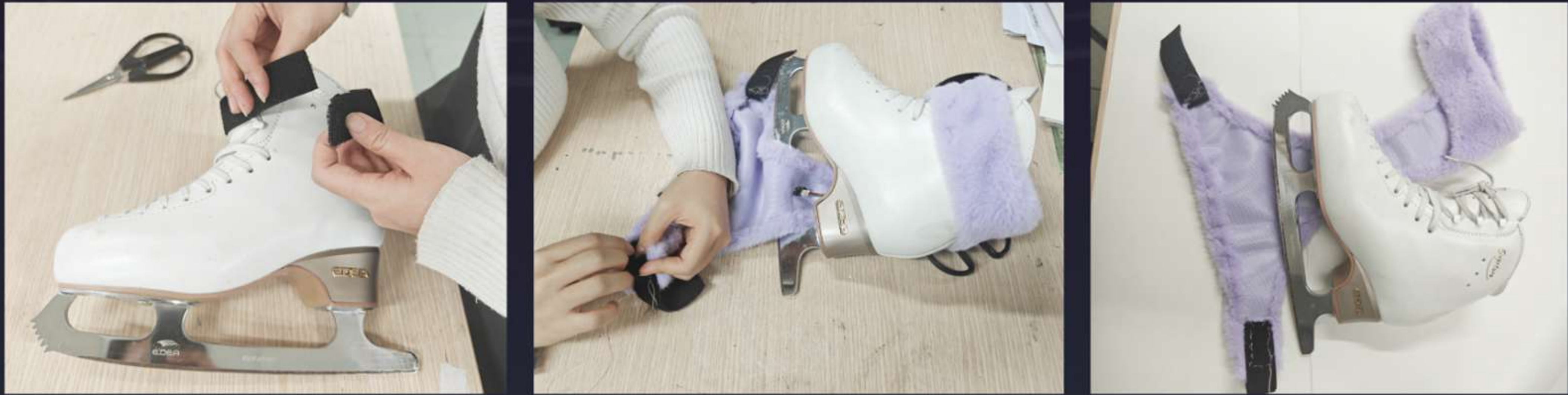
I added hook-and-loop fasteners to the sewn prototype to ensure it could be easily put on and taken off during practice, and the elasticity allowed the product to remain flexible without restricting movement
